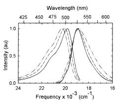
**Figure 3.** Room-temperature excitation (left) and emission (right) spectra of acridine orange in various solvents: water (dot-dashed), 3:1 glycerol-buffer (dashed), and intercalated in DNA in 3:1 glycerol-buffer (solid). The excitation maximum and Stokes shift show a clear sensitivity to the nature of the environment.
