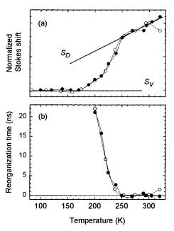
**Figure 6.** (a) Stokes shifts in DNA ( $\bullet$ ) and in a glycerol-buffer mixture ( $\bigcirc$ ) normalized to the magnitude of the transition region, suggesting that the reorganization rates are similar in both. (b) Calculated reorganization times including corrections for variations in the fluorescence lifetime, confirming that the reorganization in DNA and in solution are indistinguishable.
